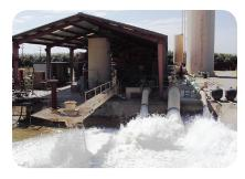
Our large volume test facility is located in Porterville, California. This facility is one of the world's largest volumetric test facilities owned by a meter manufacturer, and it offers accuracy and calibration tests of flow meters from 3 to 72-inch diameter, with flow rates up to 60,000 gpm.
