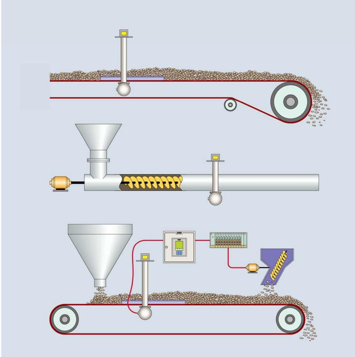
The entire system is mounted external to the conveyor and can be installed by simply bolting the frame around the conveyor, without the need to make any costly modifications to the conveyor itself. The lightweight, compact design enables it to be located in areas where space is a limitation and without the need for additional supports or foundations.
